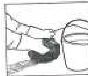
Brush the weld with a dampened stainless brush or dampened stainless wire wool
